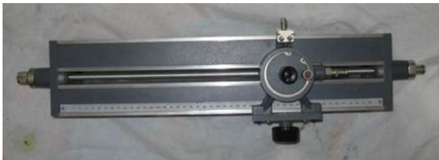
Figure 16.7: A slotted-line instrument which consists of a coaxial waveguide with a slot opening at the top to allow the measurement of the field strength, and hence, the voltage standing wave pattern in the waveguide (Figure by: Microwave101.com).
