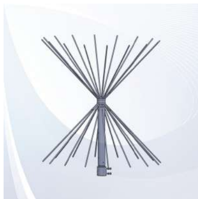
Figure 28.10: A bicone antenna can be thought of as a flared transmission line with gradually changing characteristic impedance. This enhances impedance matching and the radiation of the antenna (Figure by: antennasproduct.com).
