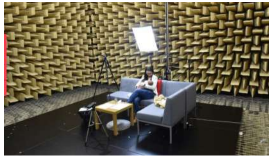
Figure 37.7: An acoustic anechoic chamber. In such a chamber, there is no reflection from the walls of the chamber; even the sound of a baby breastfeeding can be heard clearly (Figure by AGH University, Poland).
