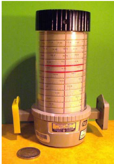
Figure 25.19: An absorption wave meter can be used to measure the frequency of a microwave. If the microwave energy enters the cavity at its resonant frequency, strong field buildup inside the cavity causes increased loss and absorption of the microwave energy by the cavity. A dip in energy level of the transmitted signal indicates the coincidence of the resonant frequency of the microwave with the frequency of the passing microwave (Figure By: https://en.wikipedia.org/wiki/Absorption_wavemeter ).
