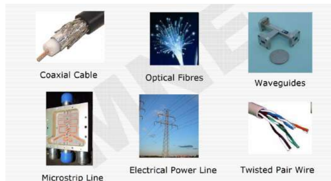
Figure 17.1: Different kinds of waveguides operating in different frequencies in power lines, RF circuits, microwave circuits, and optical fibers. Their salient physics or features can be captured or approximated by transmission lines (Figure by: Owen Casha).
