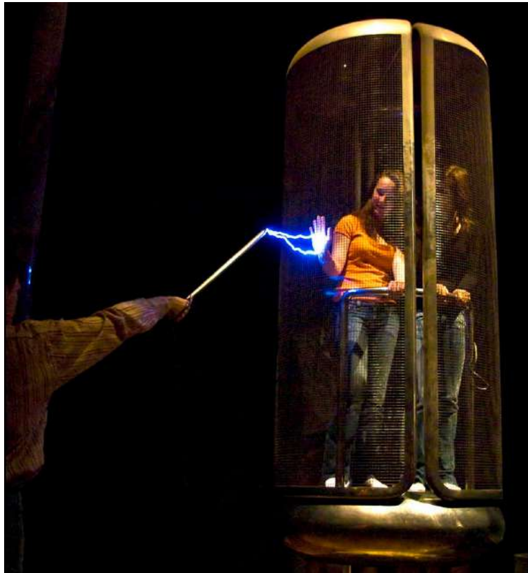
Figure 32.4: Faraday cage demonstration on volunteers in the Palais de la Découverte in Paris (Figure by: https://en.wikipedia.org ). When the cage is grounded, the potential at the surface of the cage is zero. By the solution to Laplace's equation, the potential inside the cage is a constant. Hence, the electric field inside the cage, proportional to \nabla\Phi , is zero. Charges will surge from the ground to the cage surface to ensure zero potential inside the cage. Therefore, a grounded Faraday cage effectively shields the external fields from entering the cage.
