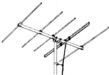
Figure 31.3: A Yagi-Uda antenna was invented by heuristics with great physical insight in 1926 even before we had computers. The principal element of the antenna is the folded dipole with four times the radiation resistance of a half-wave dipole. When an array of wire dipole antennas, each of which is less than half a wavelength, the array acts as a waveguide, or a director. When the wire antenna is slightly more than half a wavelength, the wire dipole ceases to be a waveguide, and it acts as a reflector [223]. Therefore, the antenna radiates predominantly in one direction (Figure by: https://www.wikiwand.com ).
