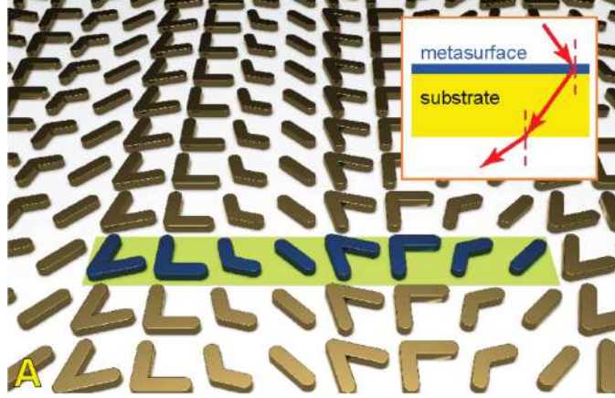
Figure 33.5: A phase screen which is position dependent can be made using nanofabrication and designed with commercial software for solving Maxwell's equations. In such a case, one can derive a generalized Snell's law to describe the diffraction of a wave by such a surface (Figure by Capasso's group [263]).
