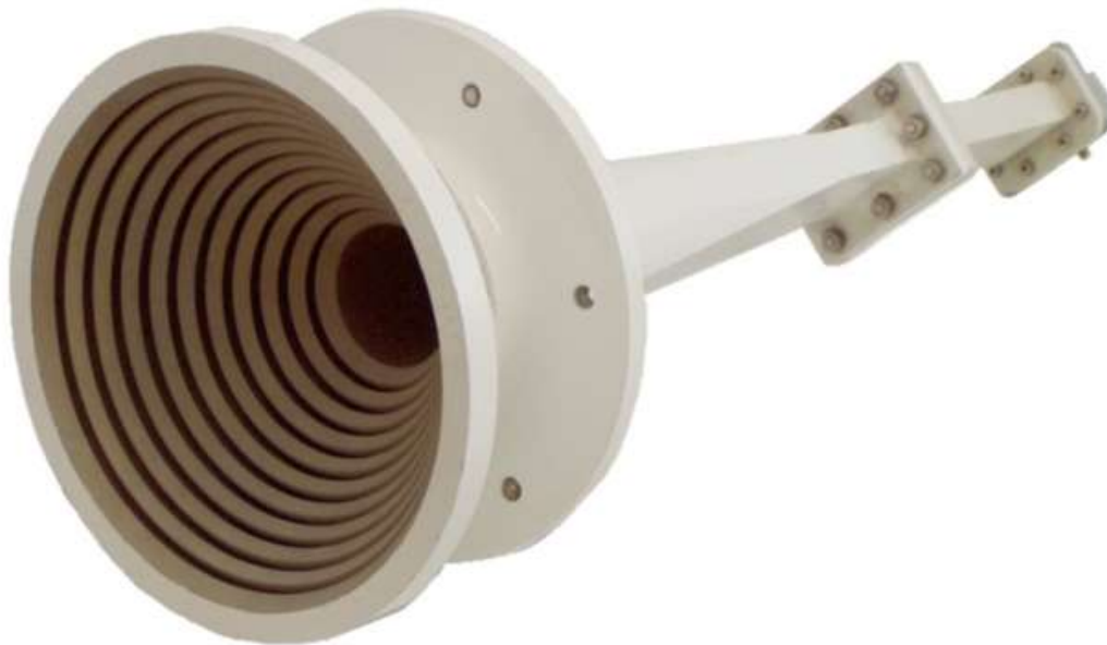
Figure 24.5: Picture of a circular horn antenna where corrugated walls are used to enhance the TE_{01} mode, which is axially symmetric. It discourages the other nonaxially symmetric modes. Therefore, the antenna has an axially symmetric field producing a radiation pattern (to be addressed later) that is axially symmetric (Figure by: Wikipedia).
