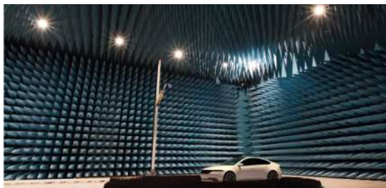
Figure 37.6: An anechoic chamber for radio frequency. In such an electromagnetically quiet chamber, interference from other RF equipment is minimized (Figure by Panasonic).
