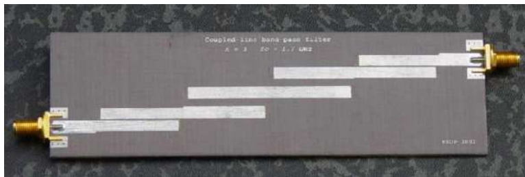
Figure 25.10: A microstrip filter designed using concatenated resonators. The connectors to the coax cable are the SMA (sub-miniature type A) connectors (Figure by agi-nas.fe.up.pt).
